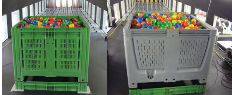
Experimental setup for measuring flow patterns of different bin designs in the ATB wind tunnel (Photo: ATB)
