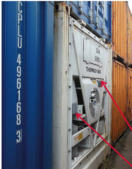
External antennas Iridium GSM GPS Location
