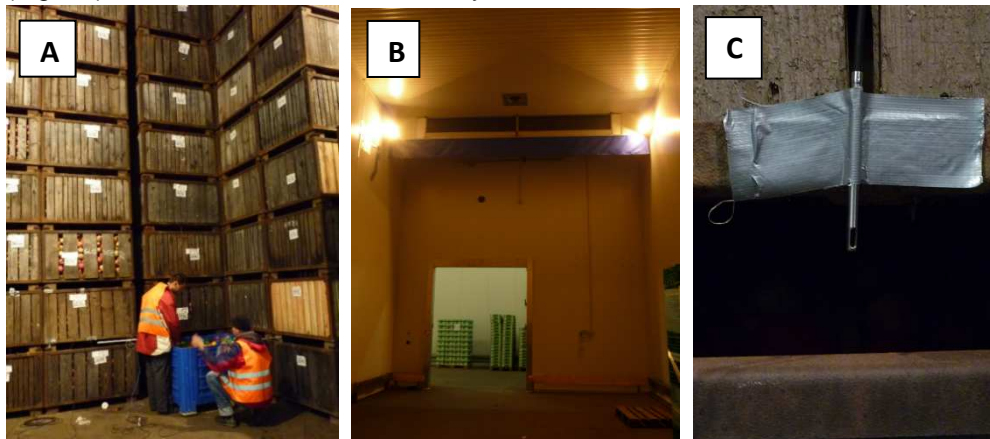
Fig. 3: Stack of apple bins in the cold store (A), cooling unit (B), airflow sensor (C)
