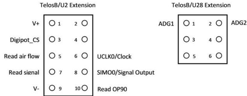
Figure 17: Pin configuration of TelosB extension U2 and U28
