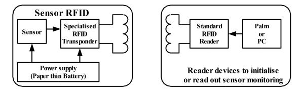
Figure 1: Block Diagram of combined RFID-Sensor-Label with Reader
